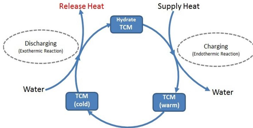
**Figure 3:** The general Aim Thermochemical Heat Storage System
