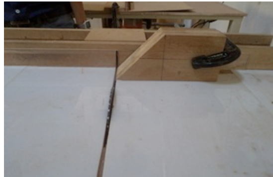
FIGURE 7: SUPPORT IN THE 45 DEGREE ANGLE CUTTING PROCESS
