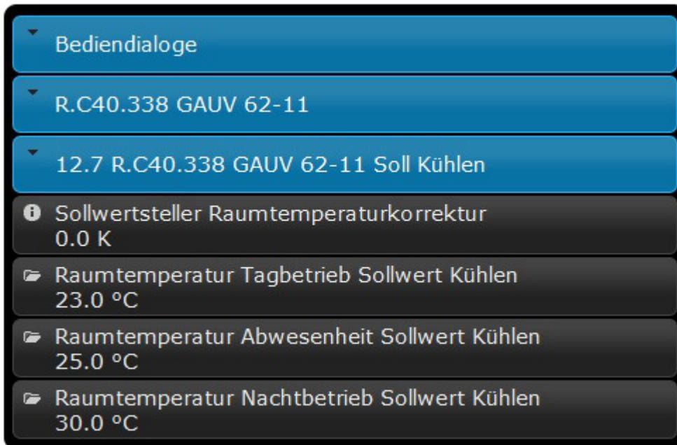
The screenshot displays a hierarchical menu structure for temperature control. The top level is 'Bediendialoge', which is expanded to show 'R.C40.338 GAUV 62-11'. This is further expanded to '12.7 R.C40.338 GAUV 62-11 Soll Kühlen'. Below this, there are several settings:
