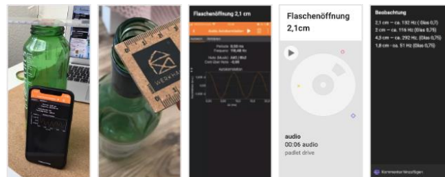
Fig. 4. Extracts from the virtual bulletin board of a group which investigated the relationship between the diameter of the bottle neck and the resulting pitch. From left to right: Picture of the experimental setup, visual documentation of the independent variable (bottle neck diameter), screenshot of the measurement (dependent variable: pitch), audio recording of the pitch and written summary of the measurement results.
