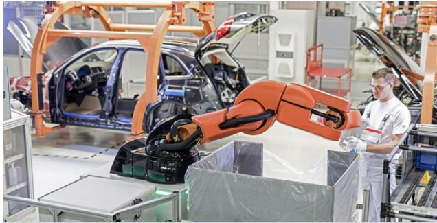
Audis collaborative robots in Ingolstadt, the “Cobots” pick up components and pass them to workers (02/2015)
