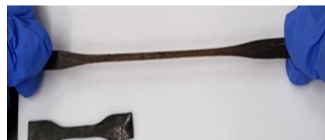
Figure 1. Dumbbell-shaped test pieces of \text{L-SO}_3\text{Na} and PDADMACI complex.
