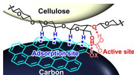
Figure 2. Schematic of cellulose hydrolysis on carbon.
