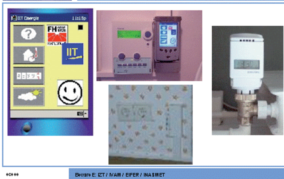
Figure 6. Display and electronical thermostat. Source: Volkswohnung Karlsruhe GmbH.
