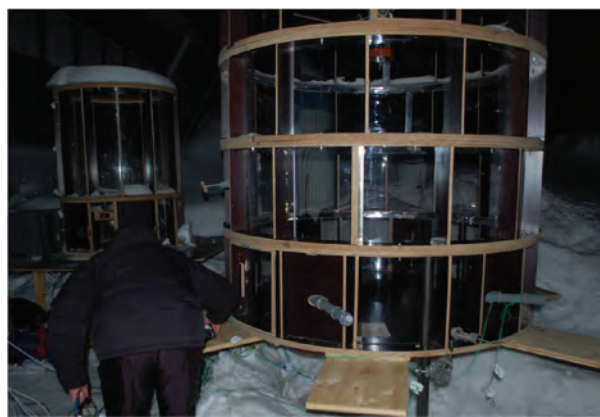
Fig. 2 – Dendrite generator snow is produced in a container
