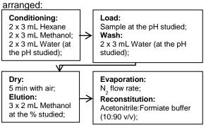
The optimization and efficiency of the extraction procedure was evaluated by calculating absolute recovery values. In order to analyze the results, a method by HPLC-FLD was developed. Separation was performed on a HPLC Prominence Shimadzu with detector RF-10AXL ( $\lambda$ ex: 230 nm,  $\lambda$ em: 312 nm). A Macherey-Nagel column Nucleodur 100-5 C18 ec (CC 125 mm x 4 4 mm d.i., 5 µm) equipped with a guard cartridge C18ec Nucleodur 100-5
