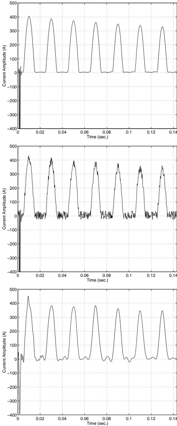
Figure 3: Real Signal. From the Top: Inrush current. Inrush current with noise in superposition. Inrush current through the denoising algorithm.
