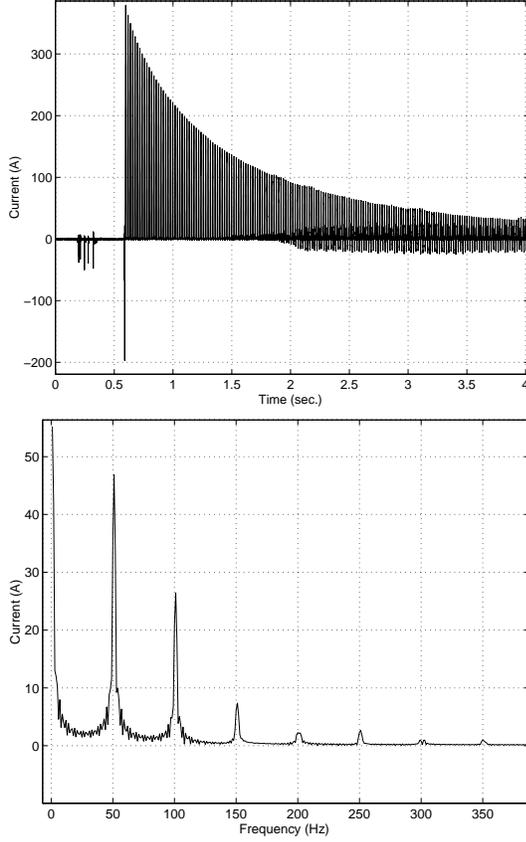
Figure 1: In Top: Inrush current: time domain. In Bottom: Inrush current: windowed spectral analysis.
