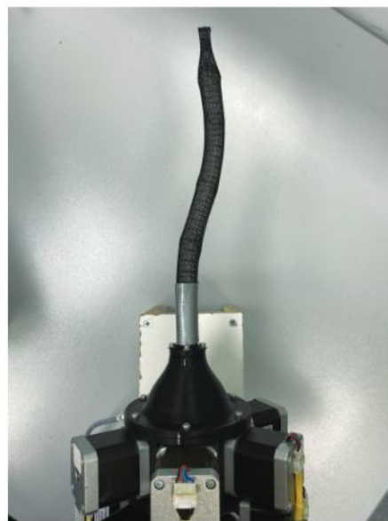
Figure 28. Pilory, a continuous hyper-redundant robot.
