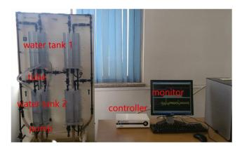
**FIGURE 17.7** The water tank experiment setup.
