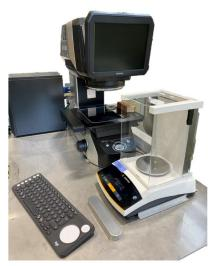
FIGURE 4.10 Quality measuring setup including a scale to measure the parts' weight and a digital measurement projector to measure the parts' dimensions.
