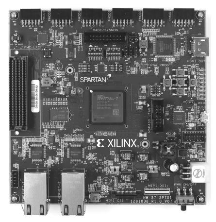
FIGURE 10.35 Spartan-7 SP701 Evaluation Board [30].
