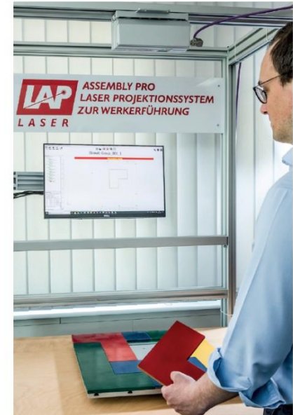
Assembly workplace with laser projector
